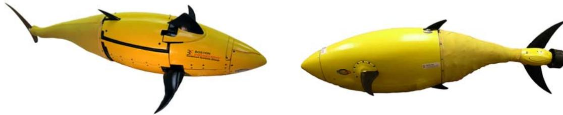
**Figure 1: GhostSwimmer™ PH I Prototypes (Propulsion Vehicle (left) and Maneuverability Vehicle (right))**
