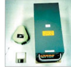
The high-precision ring-laser gyro at the core of the motion sensor. Three devices are equipped in tri-axes in the inertial navigation system.
