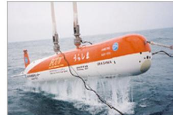
The deep-sea cruising vessel *URASHIMA* is an autonomous deep-sea exploration robot which was developed by JAMSTEC since 1998. The vehicle is able to determine its own location and follow predefined courses configured in its onboard computer. On February 28, 2005 *URASHIMA* succeeded to complete the world-record, 317-km continuous cruise.
