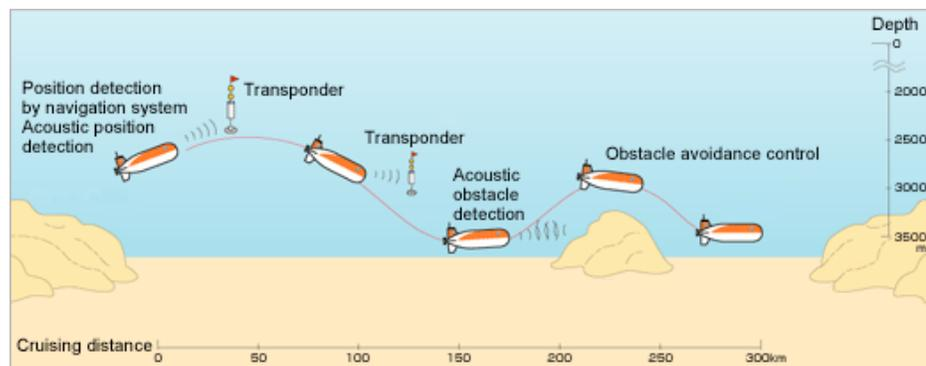
A schematic underwater robot's navigation system, which combines inertial and acoustic navigation schemes.
