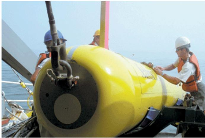
SEAHORSE 2 is being prepared for launch from the IC-508 AUV Support Vessel.
