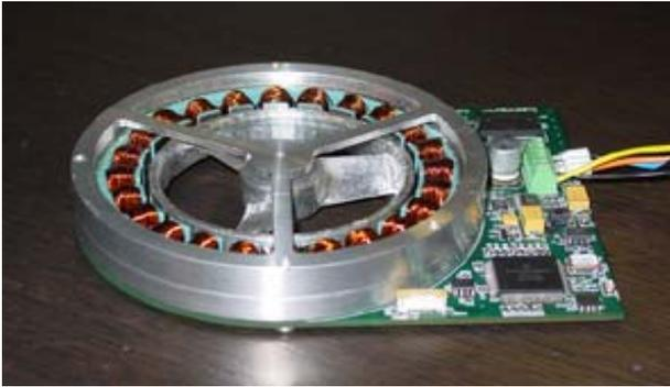
Fig. 8. Novel low-profile manoeuvring “Flat thruster” designed for high torque and low drag.
