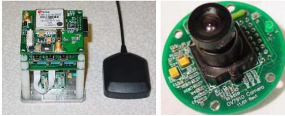
(a) Inertial plus GPS. (b) CMOS camera.
