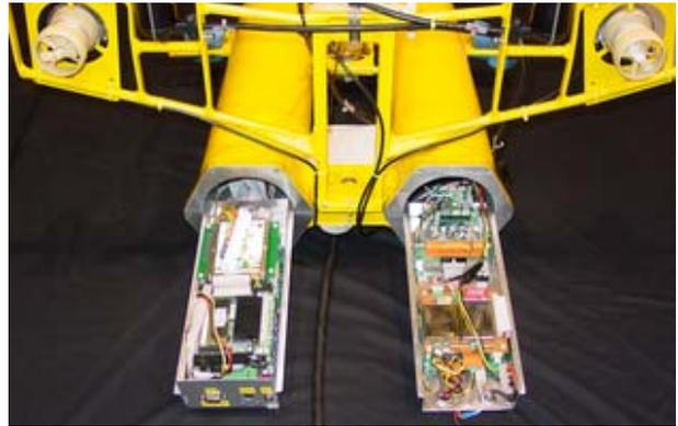
Fig. 7. Starbug's sensing and computing instrument trays.
