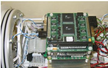
Fig. 3. PC104 stack in the internal frame.
