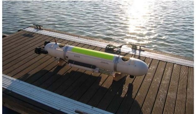
Fig. 1. MARES AUV with an external CTD.
