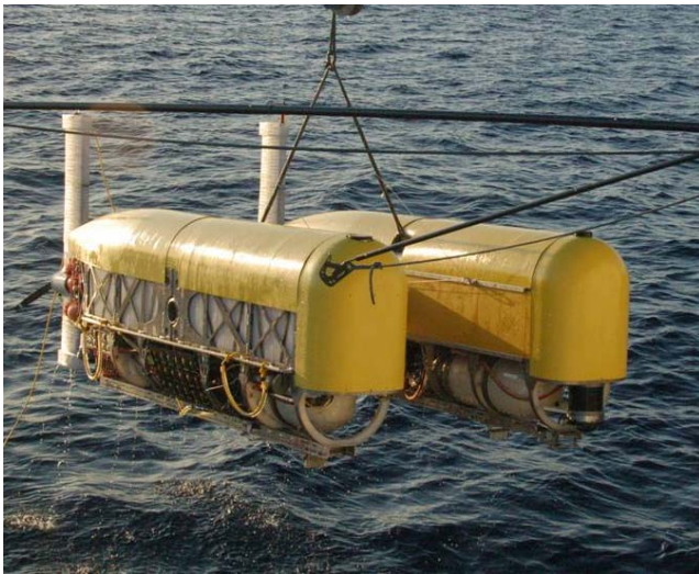
Fig. 2. The Nereus hybrid remotely operated vehicle, shown during its first engineering sea trials in the Pacific in November 2007, is designed to operate in two modes to depths of 11,000m. Left: Nereus configured for autonomous vehicle survey operations. Right: Nereus configured with a light fiber optic tether, a robot arm, sampling gear, and additional cameras for teleoperation of close-up imaging, sampling, and manipulation missions.
