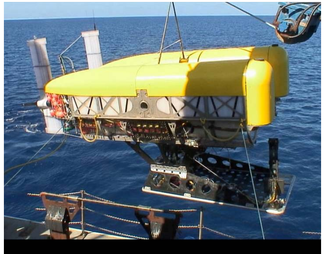
Fig. 2. The Nereus hybrid remotely operated vehicle, shown during its first engineering sea trials in the Pacific in November 2007, is designed to operate in two modes to depths of 11,000m. Left: Nereus configured for autonomous vehicle survey operations. Right: Nereus configured with a light fiber optic tether, a robot arm, sampling gear, and additional cameras for teleoperation of close-up imaging, sampling, and manipulation missions.
