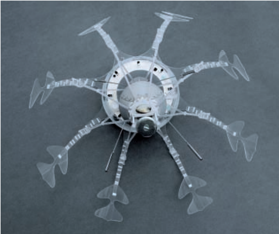
Eight Fin Ray® tentacles with rhombic joint mechanism
