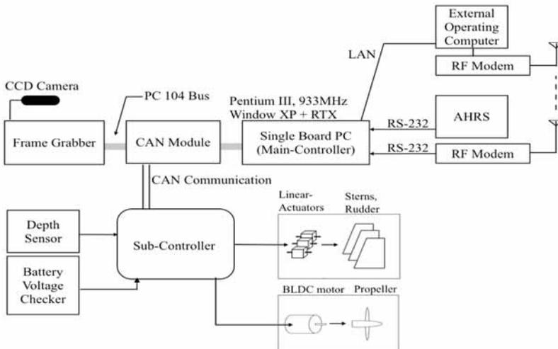
Fig. 4. Control system diagram of ISiMI.
