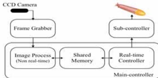
Fig. 7. Block diagram of the vision-guidance system.
