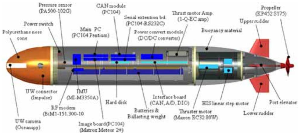
Fig. 6. General arrangement of the AUV ISiMI system.
