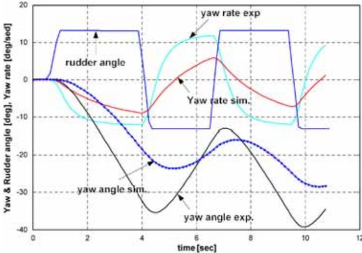
Fig. 12. Experimental results of open-loop zigzag test.
