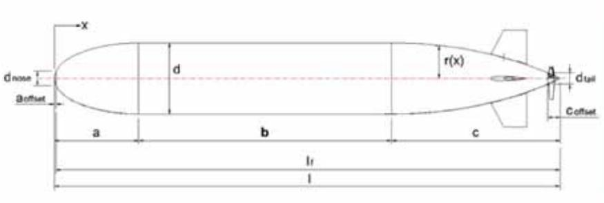
Fig. 3. Hull contour of ISiMI AUV.
