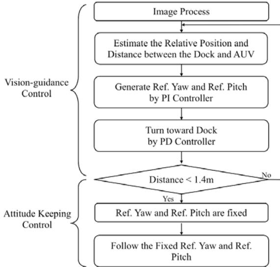
Fig. 22. Flow chart of the final approach algorithm.
