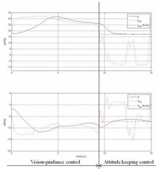
Fig. 26. Final approach: (upper) Yaw, Ref. yaw and fixed ref. yaw (lower) Pitch, Ref. pitch and fixed ref. pitch are shown respectively. After 9 seconds, ref. yaw and ref. pitch were fixed. (1)  $t = 0-9$ seconds : The vision-guidance control was applied. In this interval, all 5 lights were in the viewing range of the camera. (2)  $t = 9-15$ seconds : At  $t = 9.4$ seconds, the attitude keeping control began and the references were fixed.
