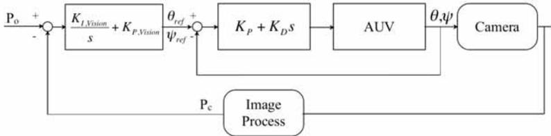
Fig. 21. The vision-guidance control algorithm.  $P_o$  is the origin of the image coordinate frame.  $P_c$  is the estimated center of the dock.  $\theta$  is pitch,  $\psi$  is yaw.  $\theta_{ref}$  and  $\psi_{ref}$  are generated reference pitch and yaw, respectively.
