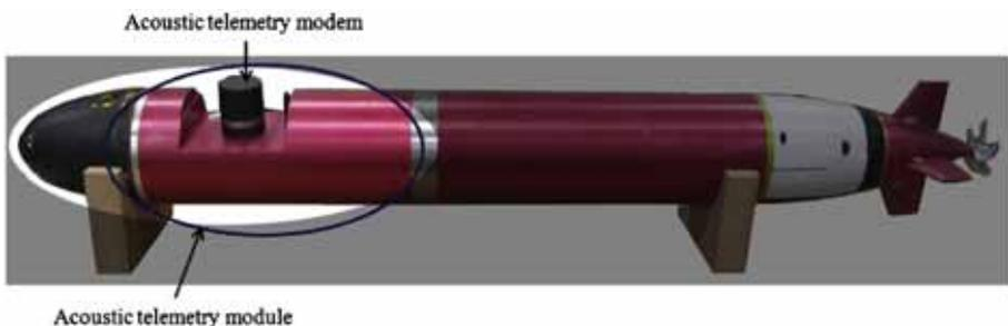
Fig. 2. Acoustic telemetry module
