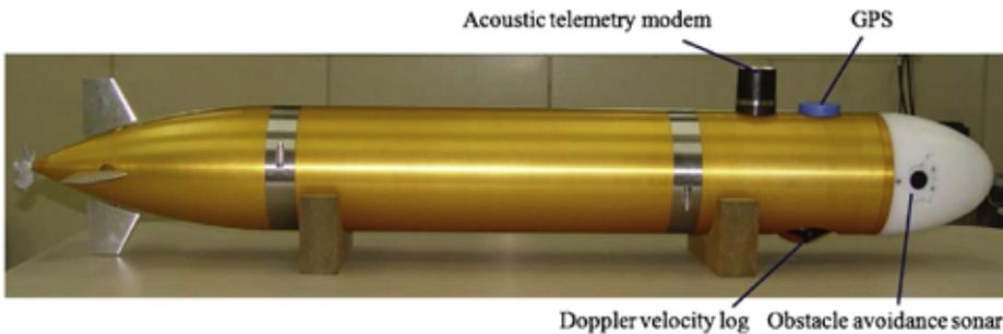
Figure 28. Sea-trial version of ISiMI AUV named ISiMI100
