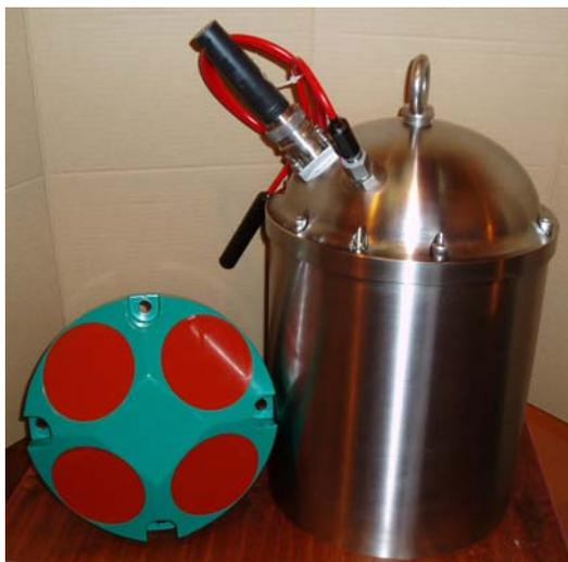
A titanium tube housing –the Inertial Navigation Unit (IXSEA-PHINS), a 300 kHz RDI ADCP, and a high performance Thales GPS receiver. We are developing navigation algorithms, involving processing of imaging or multibeam data, which, for area survey missions in deep water, will maintain GPS quality accuracy over periods of several days.
