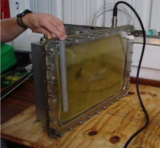
Within the each battery box are 405 Kokam Lithium Polymer cells, storing a total of 18 M joule of energy.
