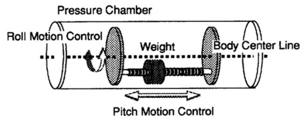
Fig. 6 Mechanism of Actuators
