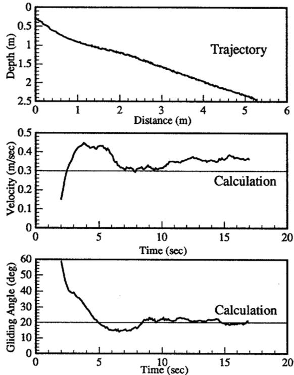
Fig. 4 Results of Gliding Experiment with a Small Model
