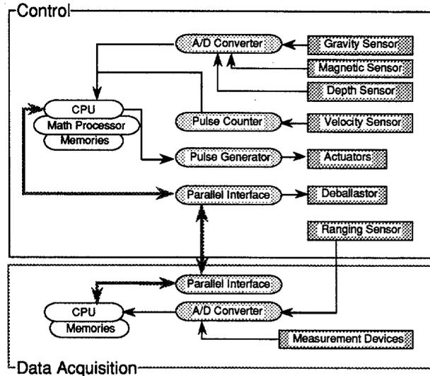
Fig. 7 Schematic Diagram of Computer System
