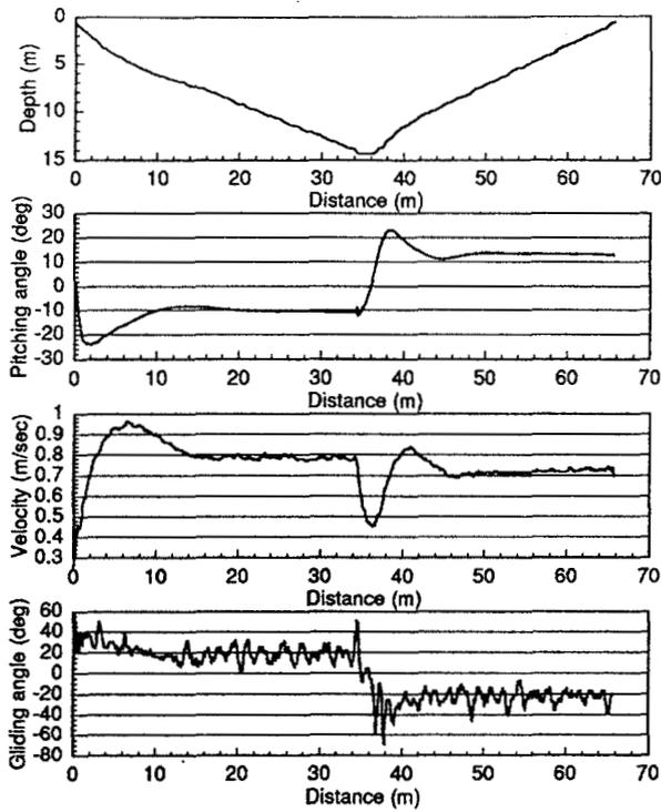
Fig. 8 Results of Gliding Experiment of 0.4788L Longitudinal C.G. Location
