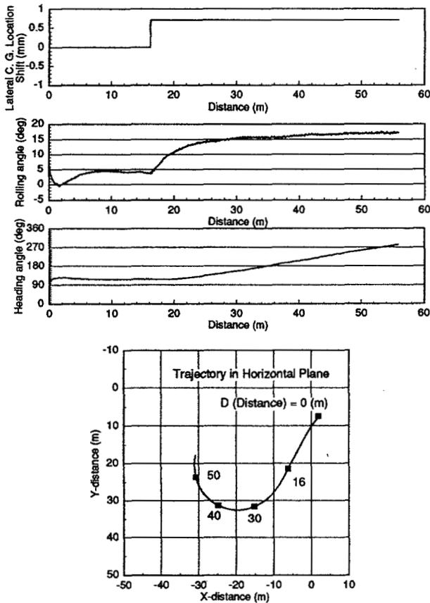
Fig. 10 Results of Step Response Experiment in Lateral Motion
