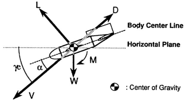
Fig. 3 AUV in Gliding
